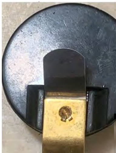
After 5 miles. Note that about 3/4 of rivet is missing.
